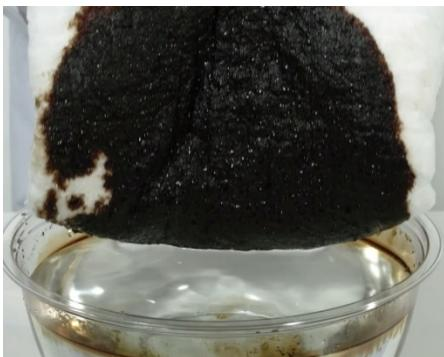
MAGIC FIBER is a cotton-like material composed of extremely thin fibers several nanometers in diameter, but it has excellent characteristics of adsorbing oil but not absorbing water. Magic fiber was greatly utilized for oil treatment work in the oil spill accident caused by the heavy rains in northern Kyushu in August 2019, and the oil spill caused by the cargo ship stranding accident in Mauritius islands in August 2020.
